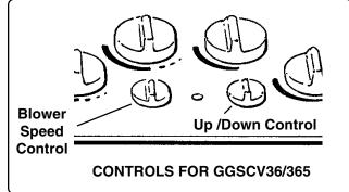
The control knob does not have to be turned OFF manually before the vent intake is lowered. It turns OFF automatically when the Vent DOWN control knob is turned towards the down position. If the control knob is not turned off, it will automatically be ON the next time the intake is fully raised.
